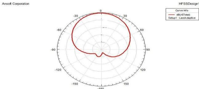
Fig. 4. Radiation pattern of the proposed antenna
