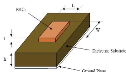
Fig. 1. Basic microstrip patch antenna structure
