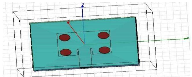
Fig. 2. Microstrip antenna with EBG Structure
