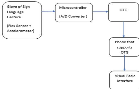
Fig. 1: Working process of sign language hand glove
