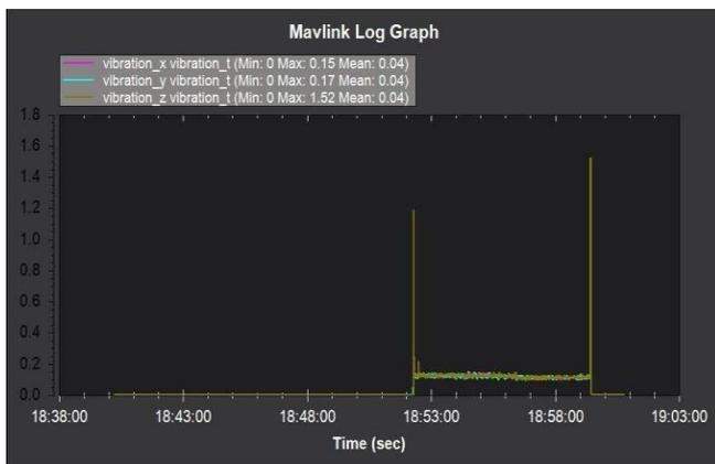
Fig. 9: Mavlink log graph to determine UAV vibration respect to X, Y, Z-axis
