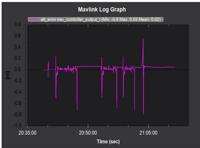
Fig. 8: Mavlink log graph to determine the attitude error in respect to Time (sec) and amplitude(m/rad)
