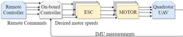
Fig. 5: Quadrotor Cascaded Control Loop Architecture
