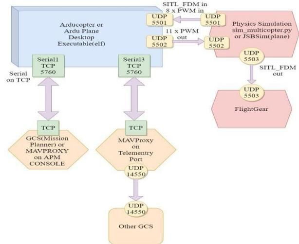
Fig. 1. Ardupilot (Software in the loop) architecture, port number may vary depending on the environment
