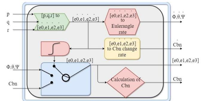
Fig. 3: Block schematics of Quaternion Angle Representation
