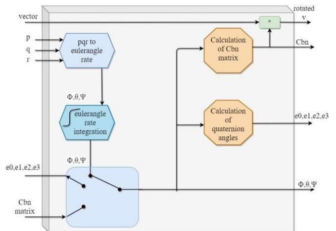
Fig. 2: Block schematics of Euler Angles Representation
