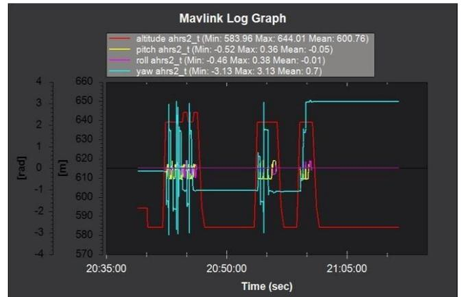
Fig. 7: Mavlink Log Graph showing altitudes AHRS (roll  $\phi$ , pitch  $\theta$  and yaw  $\psi$ ) Respect to Time (sec) and amplitude (m/rad)
