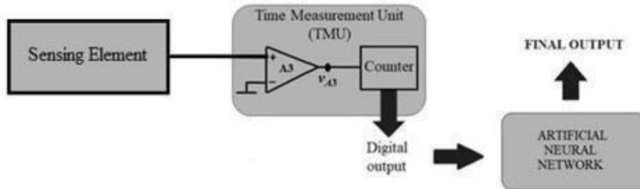
Figure 8 Basic Neural Network based Thermocouple Linerizer
