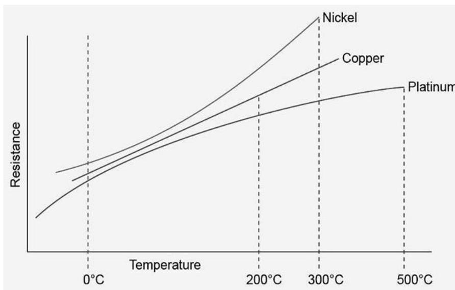
Figure 12 RTD Temperature vs. Resistance linearity
