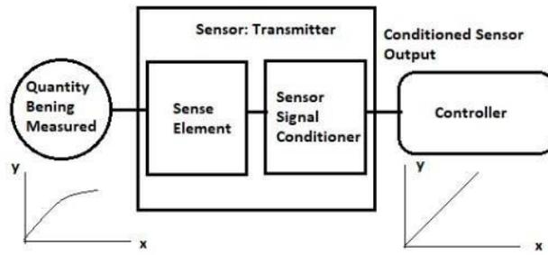
Figure 7 Basic Sensor Linearization workflow
