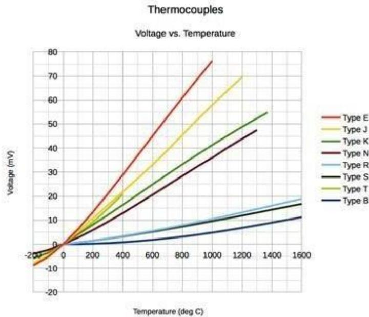
Figure 2 Thermocouple: Temperature vs. Output for each and every type
