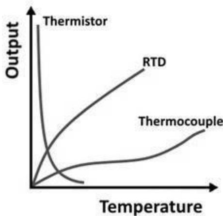
Figure 6 General Comparison between non linearity of Different temperature Sensors (Not in Scale)
