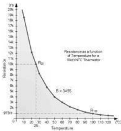
Figure 10 Thermistor non Linearity with respect to temperature
