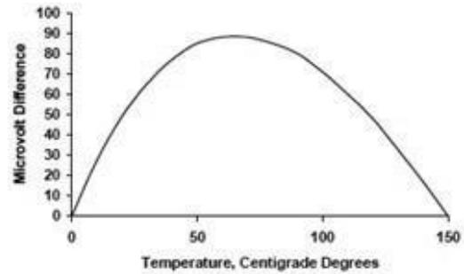
Figure 11 Thermocouple linearity range for a range of temperatures.
