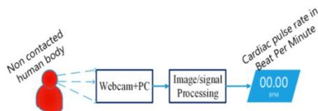
Figure 1. Principle of pulse rate monitoring system
