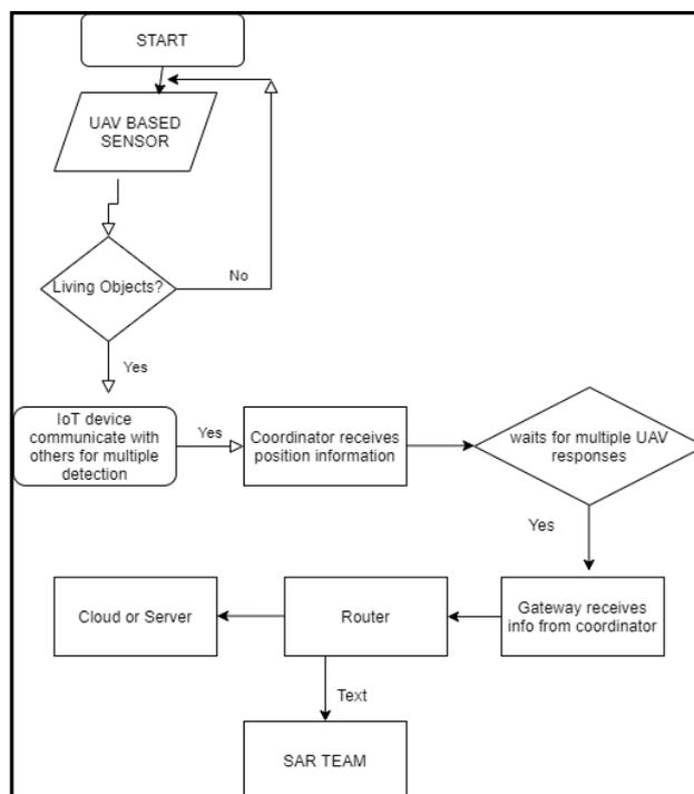
**Fig. 3. Flow Chart of proposed Model's Working Principle**
