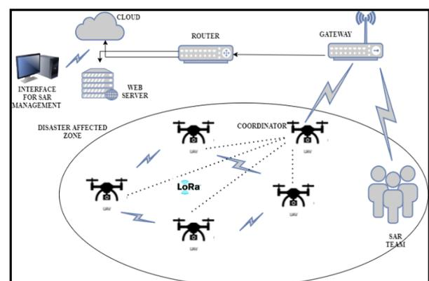
Fig. 2. IoT based Proposed Model with LoRa network for Disaster Management
